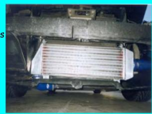
The oulet of the turbo compressor is fed to the left hand side of the intercooler via silicon hoses and aluminium piping. To do this a small section of the plastic undertray needs to be cut out to let the turbo pipe exit through and to the side of the intercooler. The blue pipe in the centre of the image is the silicon house connected to the turbo compressor outlet.
